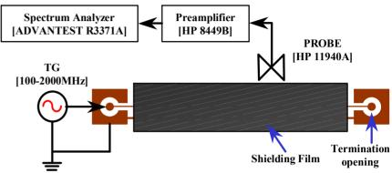
Measuring the pattern with the termination opening which marks the biggest reflected wave.
