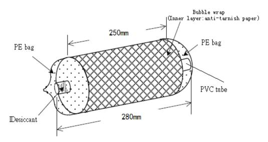
PVC tube Spec: Inner diameter: 6", Thickness: 3.5mm, Length: 280mm
