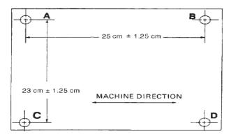
Measure the distance between hole centers A-B and C-D, alsoA-C and B-D. (I)
