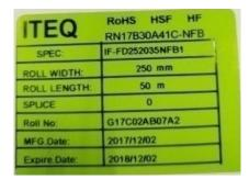
5.4 Label on Outside of PVC Tube The label shall indicate Roll No. Label Example:
