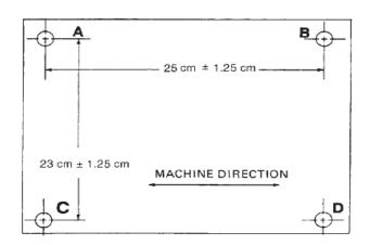
Measure the distance between hole centers A-B and C-D, alsoA-C and B-D.(I) Method B: Then etch the specimen, wash the specimen with water completely, dry . At 23  $\pm$  2 °C and 55  $\pm$  5% RH, Let stand for 1H and test in this environment.A-B and C-D, also A-C and B-D.(F1)Calculate the dimensional changes as formula 1.
