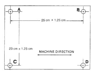
Measure the distance between hole centers A-B and C-D, alsoA-C and B-D.(I) Method B: Then etch the specimen, wash the specimen with water completely, dry. Then remeasure the distance between hole centers A-B and C-D, also A-C and B-D.(F1) Calculate the dimensional changes as formula 1.
