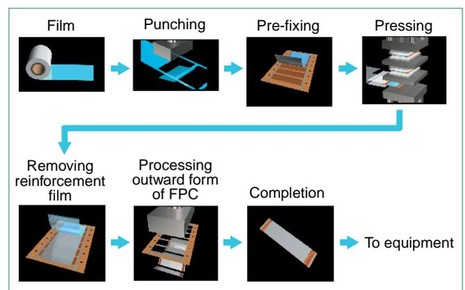
Fig. 9 Example of processing process for SF-PC1000
