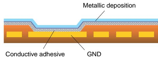
**Fig. 2 Shielded FPC (Single-sided shielding)**
